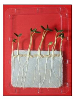
Rapid and user-friendly phytotoxicity tests with direct root/shoot length measurements by image analysis
