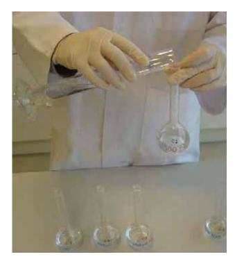
TRANSFER THE 50 ML EFFLUENT FROM THE GRADUATED CYLINDER TO FLASK C2 AND SHAKE THOROUGHLY
