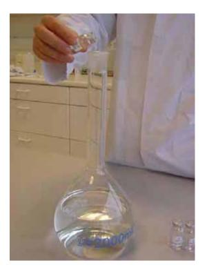
POUR THE 4 VIALS WITH CONCENTRATED SALT SOLUTIONS IN <u>+</u> 1 LITER DISTILLED WATER, IN THE 2 LITER VOLUMETRIC FLASK
