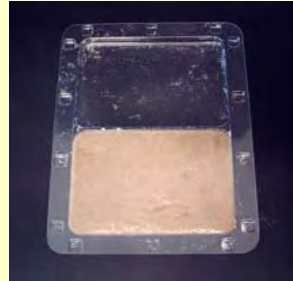
Filling of lower half of test plate with soil, and hydration
