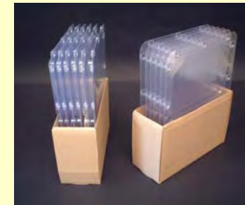
Vertical incubation of test plates in holders
