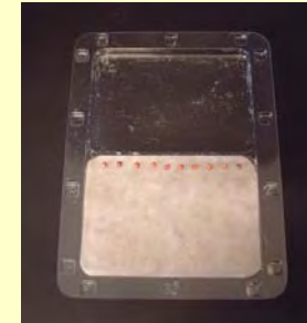
Placing of filter paper and seeds and closing of test plate with cover
