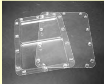
Flat transparent test plate with cover (18 x 12 x 0.8 cm)
